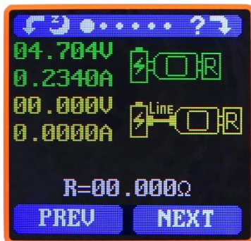
Data Connection Cable Impedance Measurement Interface
